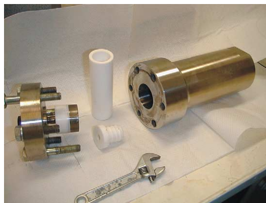
Fig. 1. Steel autoclave with a Teflon reactor vessel (white cylinder) used for experiments with ^{238}\text{Pu} -doped ceramic sample at the V.G. Khlopin Radium Institute.
